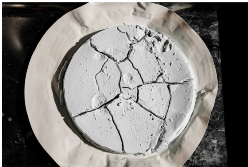
Figure 10: First mixed rare earth carbonate (MREC) produced from the Makuutu plant
